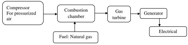
v) Flow char showing the transformation of energy in the power plant is as follows:
